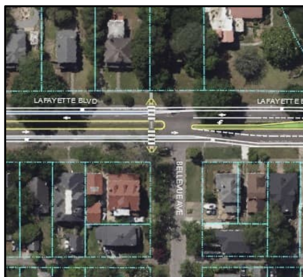
Figure 26: Proposed Intersection Improvements at Bellevue Ave
