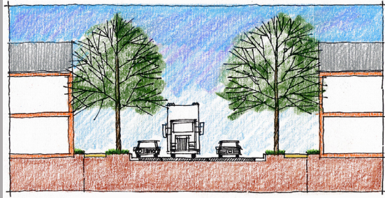
Wilson Road: Two Lanes and one Parking Lane with minimum building setback.
