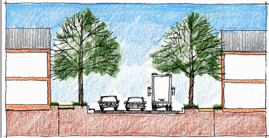
Wilson Road: Two lanes with turning lane and minimum building setback.
