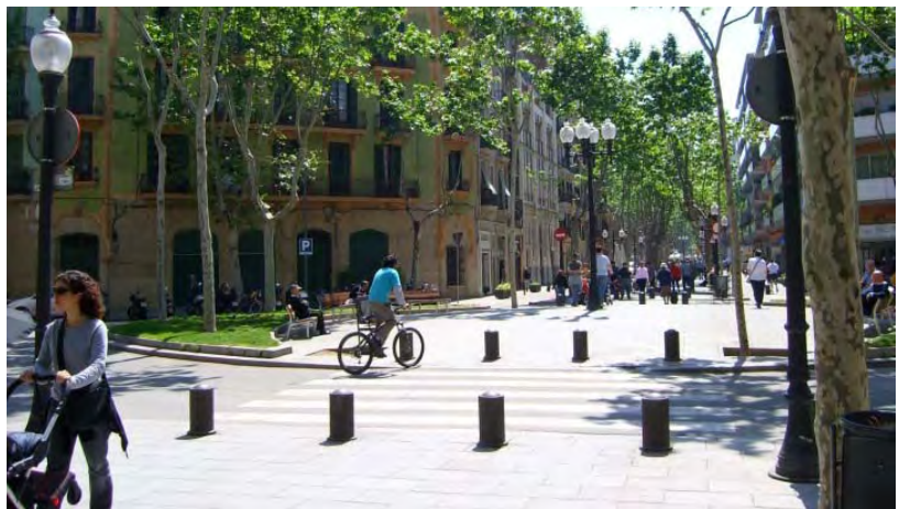
Bollards accommodate pedestrians, bikes and emergency access while restricting car access.
