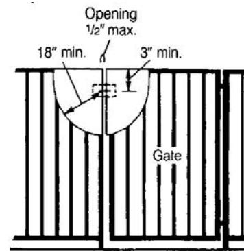
The release mechanism shall be located less than 54" from the bottom of the gate.
