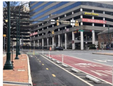
Wheel stops on a buffer with flex posts
