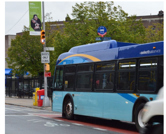
Queue jumps and transit signal priority are two types of targeted transit priority elements that can be implemented at high congestion spots along a corridor. Queens, New York. Image Source: NYCDOT
