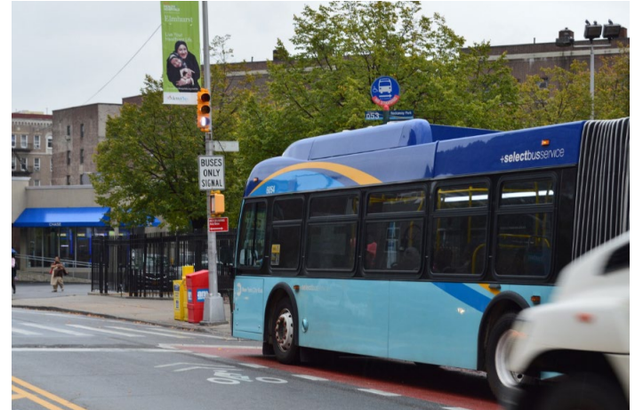
Queue jumps and transit signal priority are two types of targeted transit priority elements that can be implemented at high congestion spots along a corridor. Queens, New York. Image Source: NYCDOT
