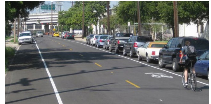
A shared lane design approach is where bicyclists share a lane with motorized vehicles. Shared lanes may have shared lane markings, also called “sharrows.” Shared lane markings are not considered to be a bicycle facility; they are a pavement marking. Austin, TX. Image Source: NACTO
