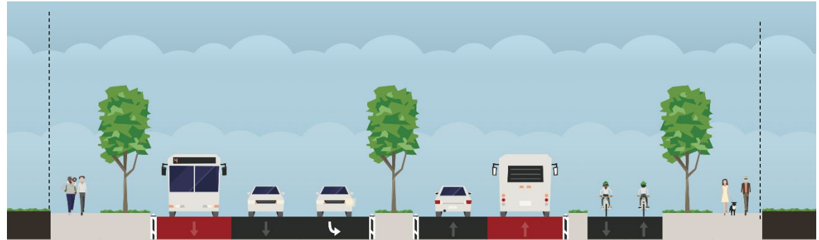
Several preferred design approaches may result from Step 2b: Determining the Design Approach. This illustration shows an example of a long-term or vision design approach for a multimodal corridor that requires additional right-of-way to provide dedicated bus lanes and separated bicycle facilities.
