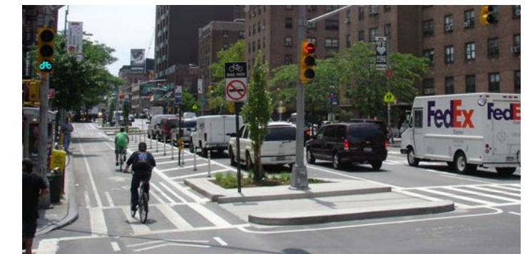
Separated bicycle lanes are separated from vehicle travel lanes by vertical elements such as curbs, planters, bollards, flexible delineators, or parked cars. New York City, NY. Image Source: NACTO
