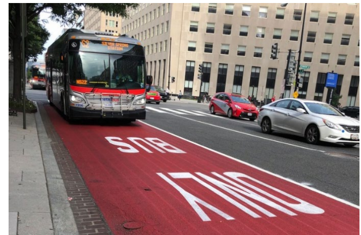
Dedicated transit lanes provide a separate lane for buses throughout an entire corridor. This approach gives the biggest boost to bus performance, but requires the most space within the cross-section. Washington, D.C.. Image Source: NACTO
