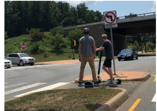
Intersections with actuated pedestrian phases and median refuges should have push-buttons in the median to prevent pedestrians from becoming stranded in the median.
