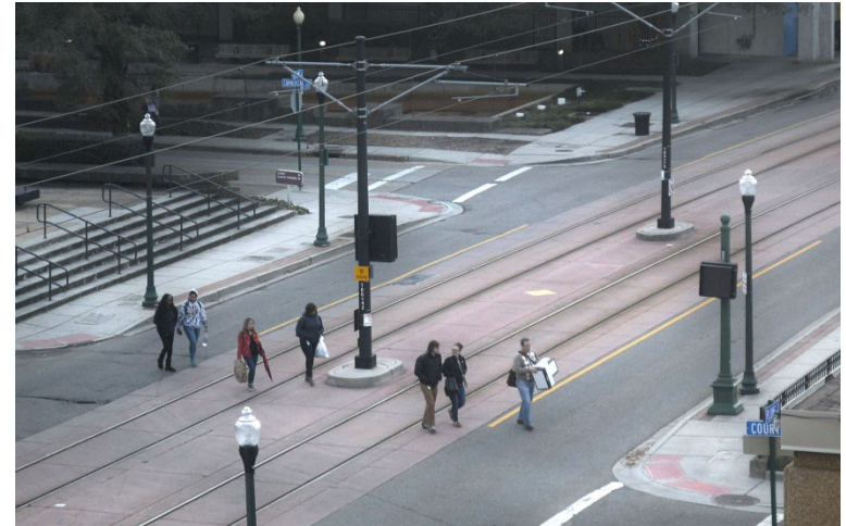
Midblock pedestrian crossings should be considered when the distance between pedestrian crossings at intersections exceeds 660 feet.
