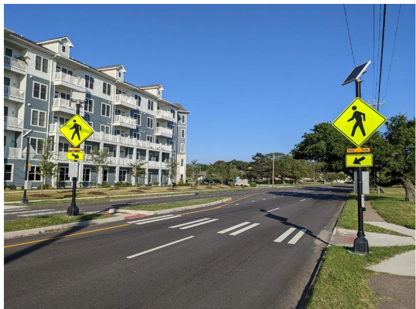
Figure 29: Rectangular Rapid Flashing Beacon (RRFB)
