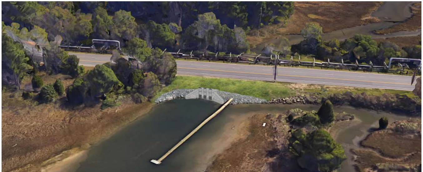
FIGURE 5-15: JEB Little Creek – Tide Gate Concept Design
