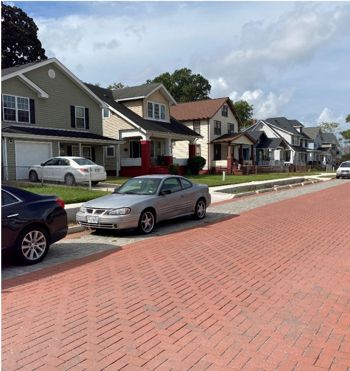
Permeable pavers, such as these in Chesterfield Heights, can help reduce impervious surfaces and stormwater runoff (WRT)
