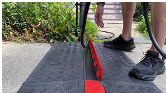
Figure 32. EV cable protector
